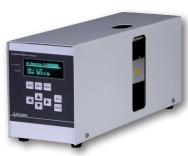
Flash10 detector is designed for preparative and flash applications, with four continuously variable wavelength in the range 200-400nm, 200-600nm and 190-840nm for each instrument. Noise level at 254 nm are  $\pm$  5 x 10-5 AU with an empty cell. Detector has analog output.
