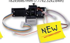
\* Detector uses one new control board which replaces two boards used in previous detector types
