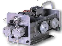
OEM preparative pumps suited for preparative and flash applications. Controlled by RS232. With pressure sensor. IOTA50 50 ml/min, 30 MPa (4351 PSI) IOTA100 100 ml/min, 15 MPa (2176 PSI) IOTA300 300 ml/min, 7.5MPa (1015 PSI)
