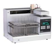
Fraction Collector EFC2096 collects fractions according to chosen method which can be created manually by keyboard just as using ECOMAC software. Analog input allows collecting based on detector signal. Racks for 9, 21 and 40 ml tubes.
