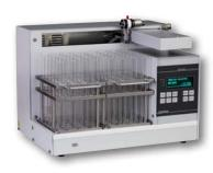
Fractions collected according to chosen method which can be created manually by keyboard, just as using **ECOMAC** software. Analog input allows collecting based on detector signal. Racks for 9, 21 and 40 ml tubes.
