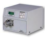
Single piston pump suited for column washing and columns regeneration process. Kappa **10PP includes pressure sensor**. It is designed with piston diameter of 1/8". Completely new concept of electronic control and drive of pump allows it to be used as a standalone unit.
